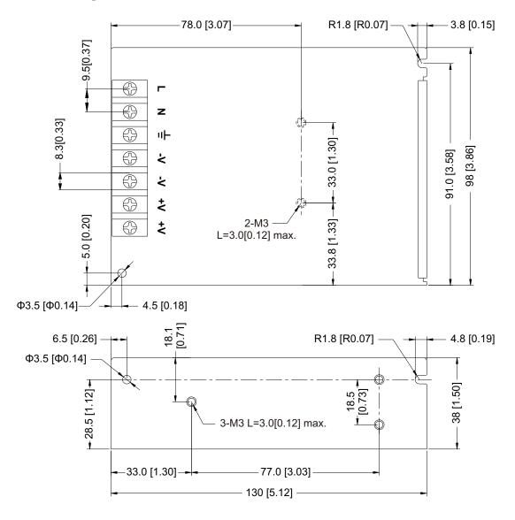
Recommended screw length is measured from the power supply surface
